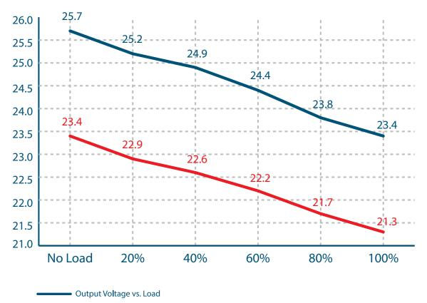
Output Voltage With a Typical Dimmer
